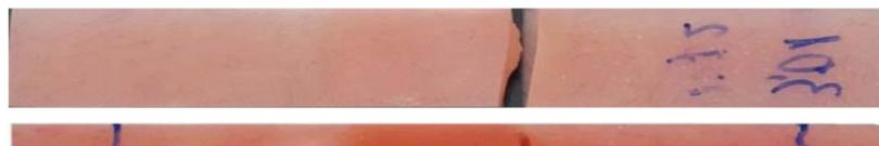
Figure 3 Illustration of mix type of failure in which fracture occurred in both repairing material and the interface.
