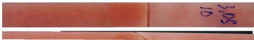
Figure 2 Illustration of adhesive failure in which fracture occurred at the interface
