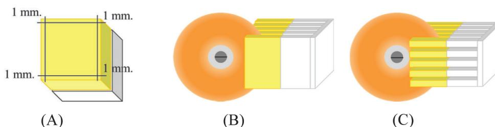
**Figure 1.** Schematic illustration of microbars preparation. (A) 1-mm peripheral rims of specimens were discarded. (B) The block was partially sectioned, leaving 1.0 mm of intact surface at the end of the block. (C) The cemented block was then rotated 90°.
