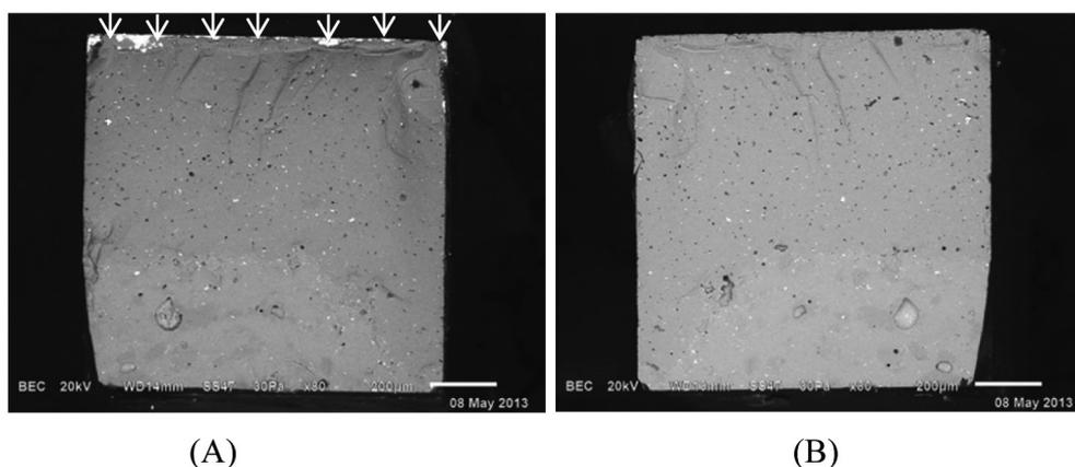
**Figure 2.** SEM image (80X) of an interfacial failure of e.max<sup>®</sup> ZirCAD/ZirLiner/ e.max<sup>®</sup> Ceram (ZLC). Fracture originated at zirconia-veneer interface, leaving exposed zirconia grains (arrows). (A) Zirconia side and (B) Veneer side
