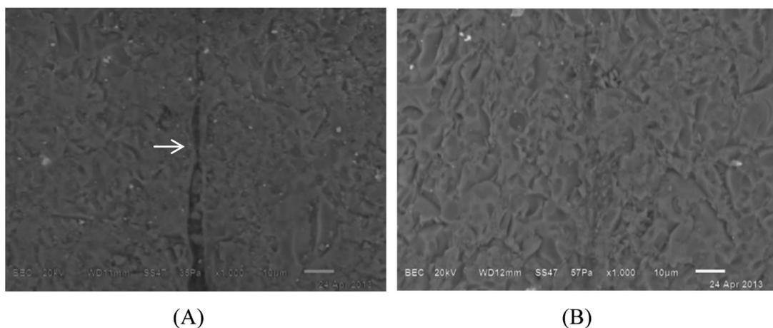
**Figure 6.** SEM image of e.max®ZirCAD/e.max®ZirPress(1000X): (A) Unblasted liner material created microgaps between e.max®ZirLiner/e.max®ZirPress. (B) Blasted liner material eliminated microgaps between two materials
