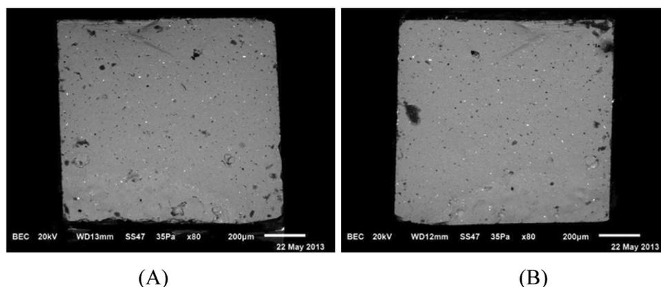
**Figure 3.** SEM image (80X) of a cohesive failure in veneering porcelain of e.max<sup>®</sup> ZirCAD/ ZirLiner/e.max<sup>®</sup> Ceram (ZLC). Fracture originated and propagated in the veneer ceramic. (A) Zirconia side and (B) Veneer side
