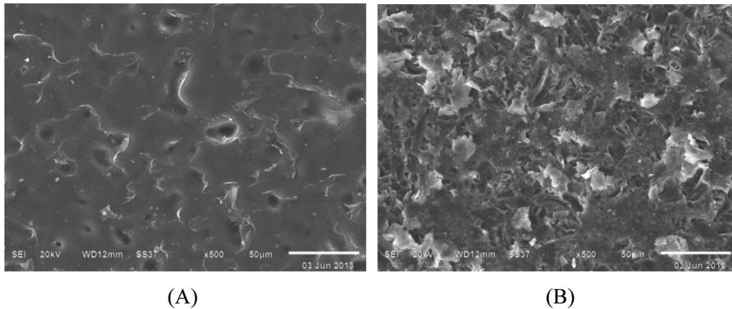
**Figure 4.** SEM images (500X) of ZirLiner surfaces: (A) Unblasted ZirLiner surface (B) The fired liner surface after sandblasting with 50-µm aluminum oxide particles
