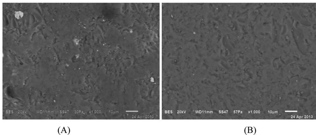
**Figure 5.** SEM image of e.max®ZirLiner/e.max®Ceram (1000X) shows good contact between the liner-veneer interface without microgaps. (A) Unblasted liner material and (B) Blasted liner material.
