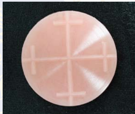
Figure 2 The specimen after removal from the mold showing two crossing triangular projections with reference points
