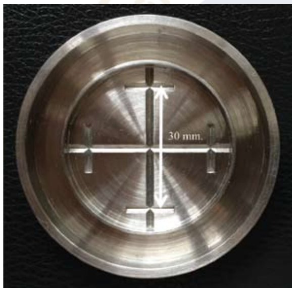
Figure 1 Circular stainless mold. (40 mm in diameter, 3 mm in thickness with 2 crossing triangular grooves)
