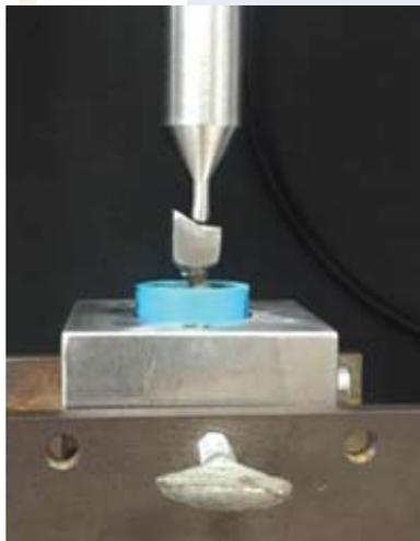
**Figure 3** Customized stainless steel cylinder rod and specimen were mounted on a universal testing machine (ElectroPuls E1000, All-Electric Test Instruments, Instron)
