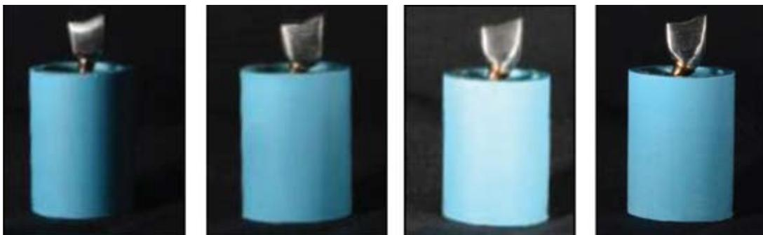
**Figure 2** Implant abutment assembly and superstructure cemented before cyclic loading
