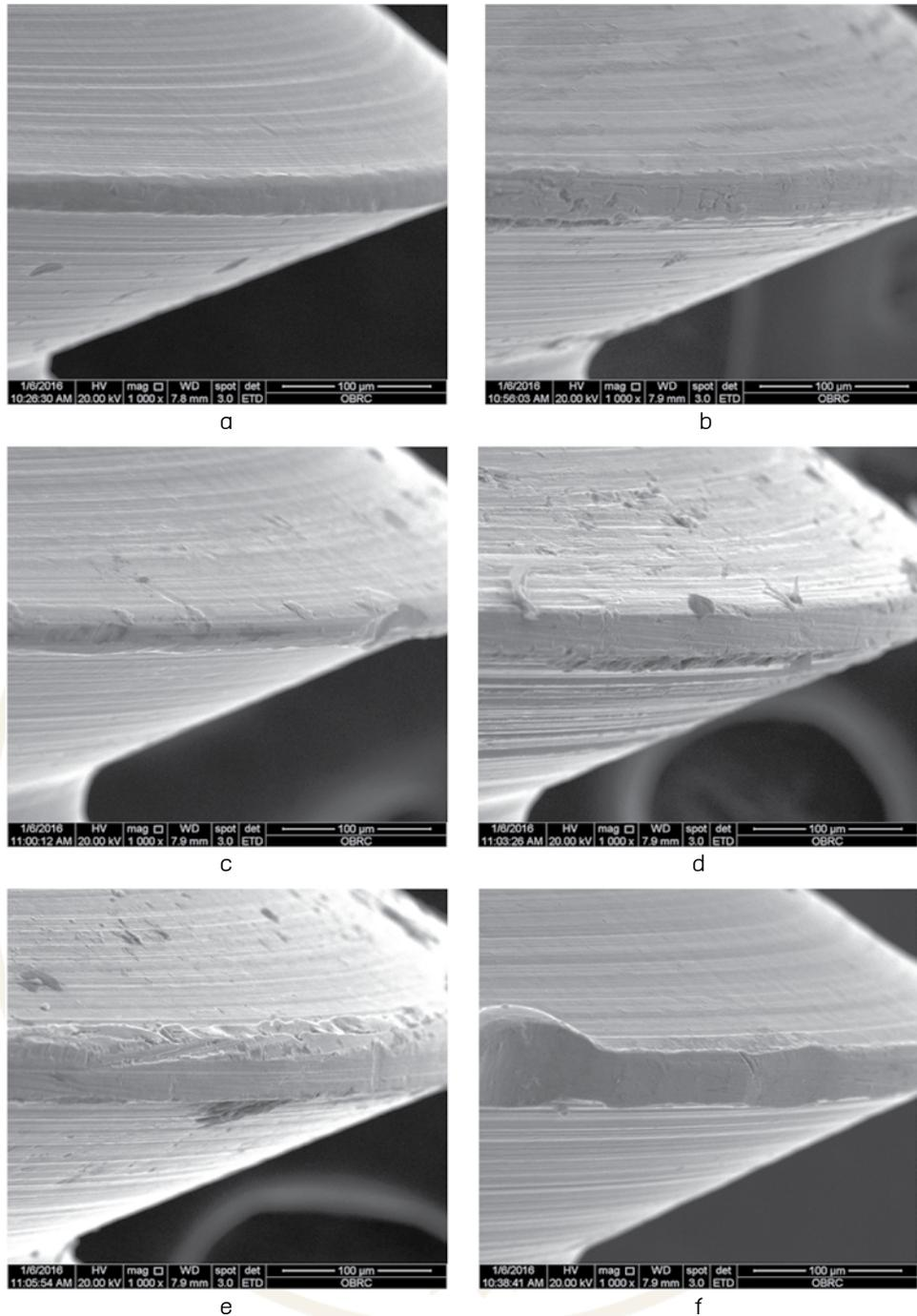
**Figure 4** SEM of the third thread of the abutment screws; (a) before cyclic loading, (b-f) after cyclic loading of groups I-IV and a fractured screw.
