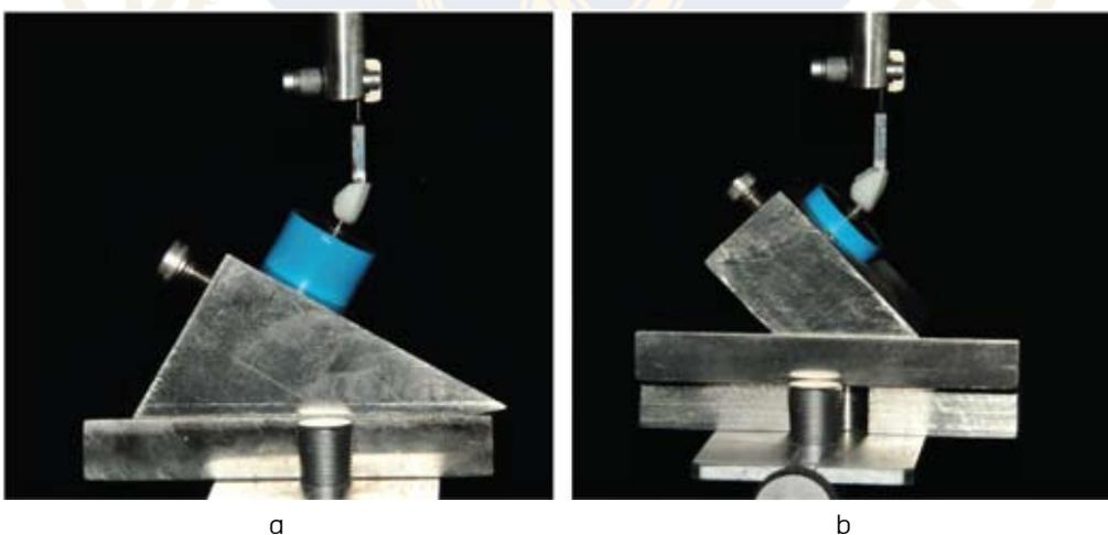
**Figure 2** The incisal edge of two wax-up teeth was cut off to create a flat surface at 30° angles to the long axis of the teeth, which was the area of loading point in both (a) straight and (b) angled abutments.
