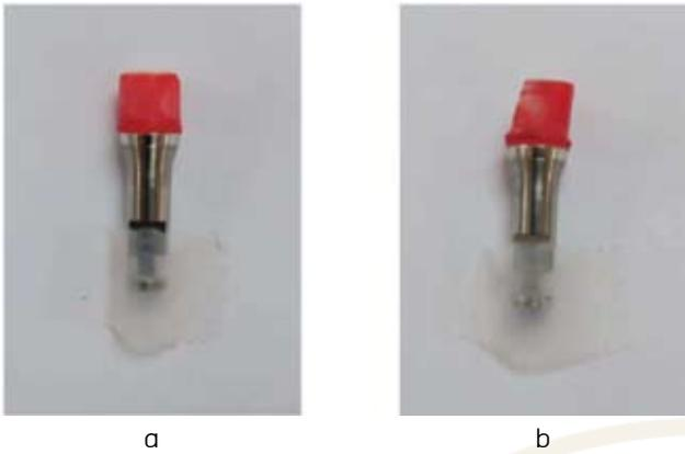
**Figure 1** Customized (a) straight and (b) angled abutment, before casting
