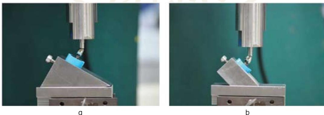
**Figure 3** (a) Groups I and III (straight abutment), the specimen was aligned into a mold which was 30° from the axial line. (b) Groups II and IV (angled abutment), the specimen was aligned into a mold at a 45° angle from the axial line.
