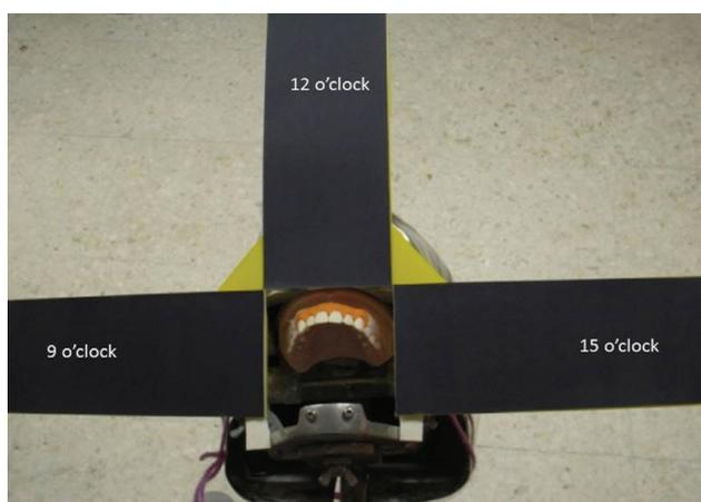
**Figure 1** Experimental upper dental cast and measuring board were secured in phantom head
