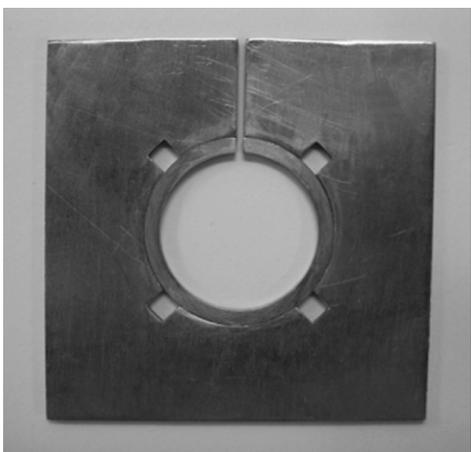
Figure 1 Mold used for preparation of water sorption specimens.
